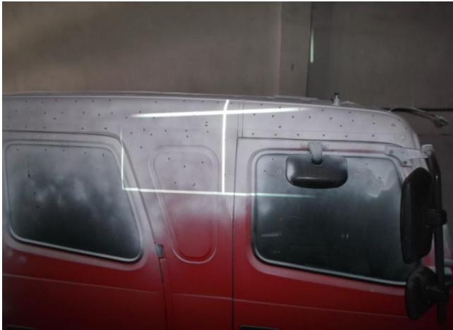
Pic. 2. Object coated with antiglare agent and positioning markers.
