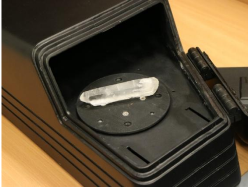
3D scanning of quartz crystal using SMARTTECH mini
