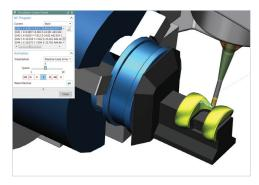
account of any program content provided by the postprocessor. Home positions, special tool change motion and other content can be inserted by the postprocessor, minimizing surprises by making sure to simulate the posted g-code.
